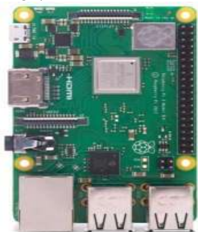
Figure 2: Raspberry Pi 3 Model B Fingerprint Sensor R-307: A noteworthy check scanner is just a sort of improvement
